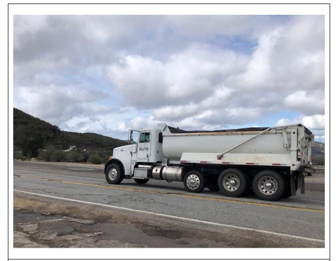
**Photo 3:** Haul trucks used for dirt export from C 440 were observed utilizing load covers to prevent dust emissions in accordance with APM AIR-02.
