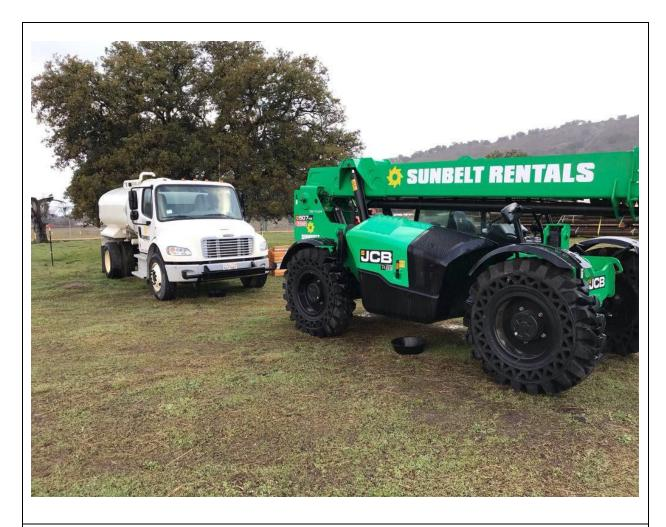
**Photo 5:** Drip pans were observed under staged equipment at Santa Ysabel Staging Yard (TL 626 Conversion North) to prevent hazardous material discharge onto the ground in accordance with the SRNP and MM PHS-2.
